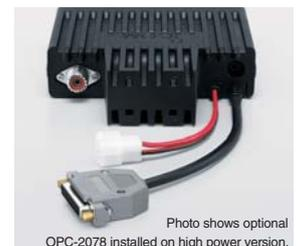
Photo shows optional OPC-2078 installed on high power version.
